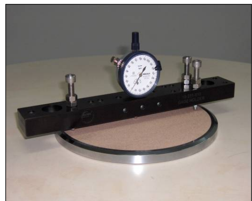
Inspection of wafer chuck's flatness 18-211-010
